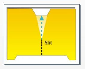
• The resistance to tearing is either factored into the equipment scale using the pendulum capacity or read from a digital display computed by the microprocessor within the instrument. The resistance is recorded as the tearing strength of the specimen
